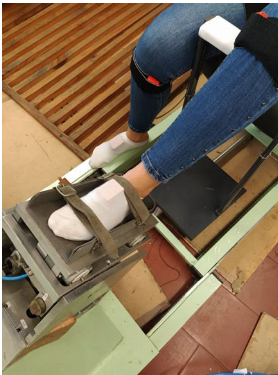
Fig. 1 XSens® sensors placed on the foot and tibia of a volunteer during testing
