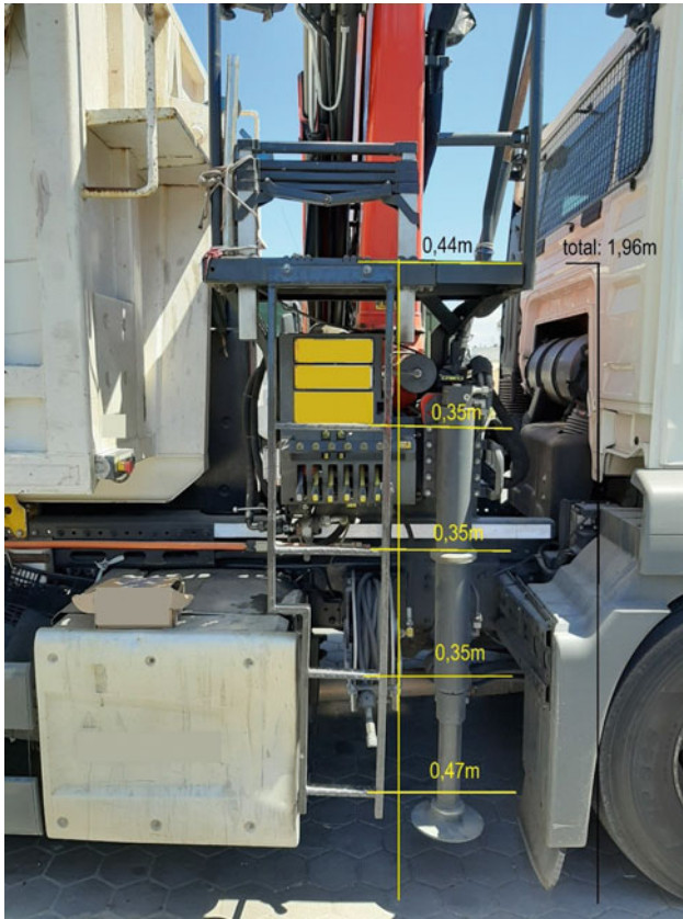
Fig. 2 Vertical ladder used to ascend and descend at each stop of Eco points
