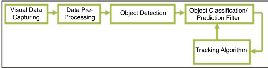
Fig. 2.4 Basic object tracking methodology
