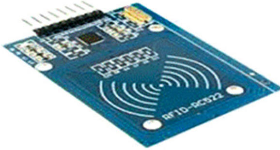
Fig. 4 MIFARE 13.56Mhz RC522 RFID card reader
