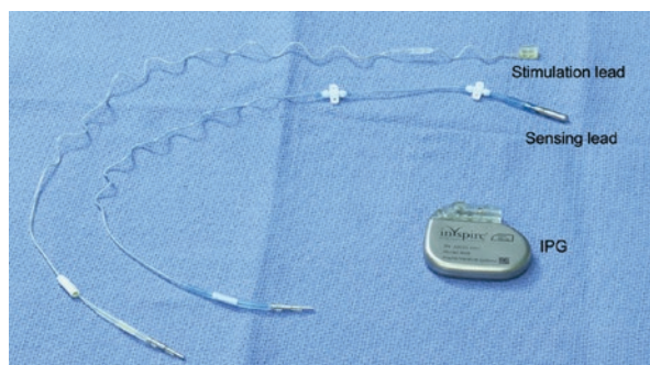
Fig. 13.1 The system consists of three components: stimulation lead, sensing lead and implantable pulse generator (including battery and a chip for stimulation)
