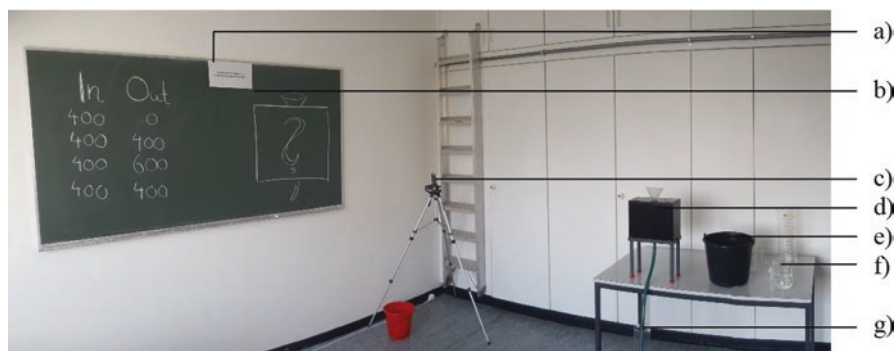
Fig. 18.1 Black box setting. Components are labelled as follows: (a) written task: participants were asked to develop a model of the internal mechanisms of the black box, (b) exemplarily labelled chalkboard, (c) video camera (1 of 3), (d) black box, (e) water reservoir, (f) beakers of different sizes, (g) volumetric flask
