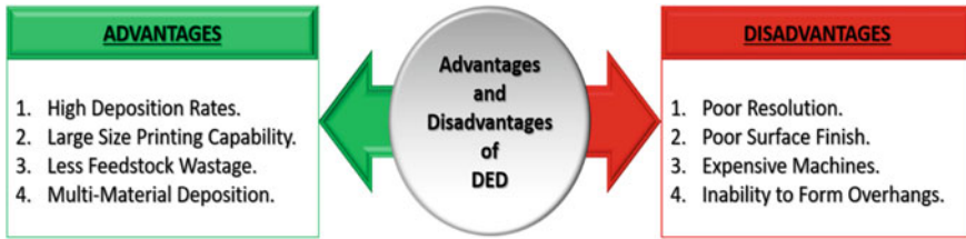
Fig. 1.14 The advantages and disadvantages of the DED process over PBF utilized to 3d print metal components
