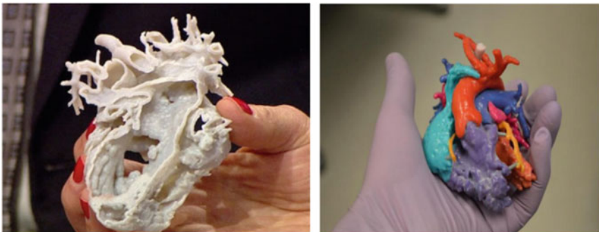
Fig. 7.4 Prototype of “Heart” using rapid prototyping [54]
