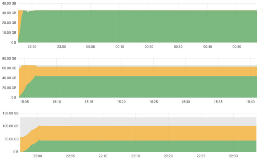
Fig. 6. Memory utilization charts for the DLRM benchmark. The green area represents the memory reserved by the benchmark, the yellow area for the memory used by the OS as a cache for IO operations (irrelevant for our analysis). From top to bottom: 1) g3s.xlarge instance with 31 Gb of RAM; 2) g4dn.4xlarge with 64 Gb of RAM; and, 3) g4dn.8xlarge with 128 Gb RAM.
