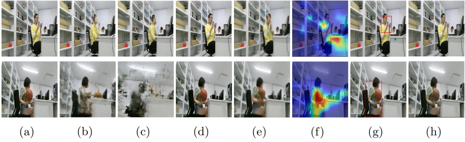
Fig. 6. Examples of the anomalies in the Robotic + (top row) and HAM (bottom row) datasets. Our method successfully detects these examples. (a) Original inputs. (b)–(e) are reconstructed images by FA-GAN, GANomaly, skip-GANomaly, and RIAD, respectively. (f) Attention maps. (g) The positions with the highest activation scores (marked as blue dots) and the nearest regions (marked as red rectangles). (h) The inpainting results from the images obtained by masking the regions in (g). (Color figure online)
