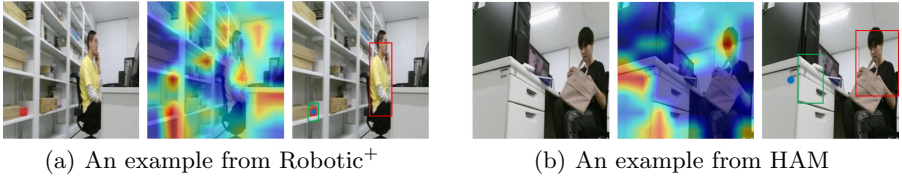
Fig. 7. False negative examples with our method in the Robotic + (a) and the HAM datasets (b). The leftmost image in (a) is the input, and the middle one is the attention map. The rightmost image in (a) shows the position with the highest activation score (marked as a blue dot), the nearest region (marked as a green rectangle), and an anomalous region (marked as a red rectangle). (Color figure online)
