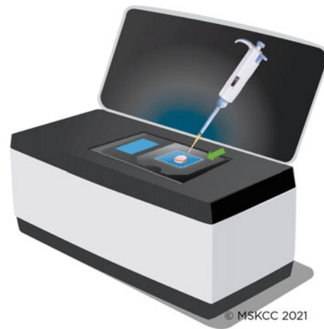
Fig. 3.4 A cartoon of the EVCM device showing tissue mounting procedure. Ex vivo tissue placed on a glass slide (green arrow) and inserted in the grooves of the EVCM device. The blue area reflection seen in the glass slide is from the blue laser light coming from the objective lens (not visible in this cartoon) underneath. Use a pipette (white arrow) to put a few drops of saline on the tissue surface
