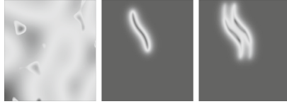
Fig. 1. The three input layers. From the left: the terrain elevation map, the trajectory centre, and the wheel trace.
