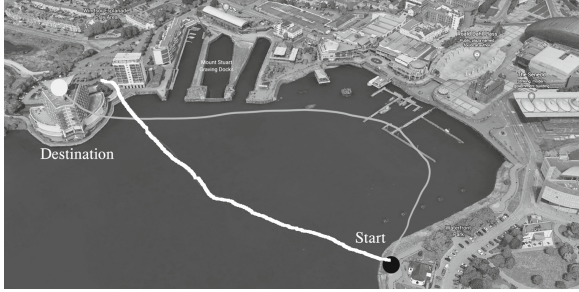
Fig. 1. A robot navigates from the start location to the destination on the left-hand side. The white trajectory is traversing in a feature-poor area, which is not suitable for SLAM-based localisation. The grey trajectory is a more preferred path, which maximises feature observations for robust SLAM-based localisation.
