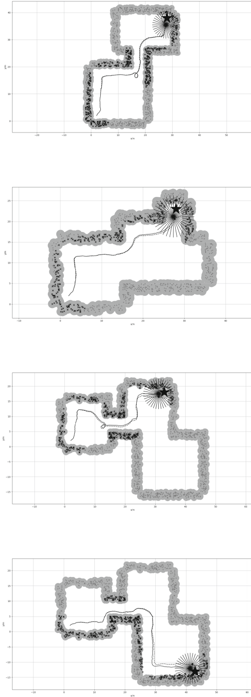
Fig. 7. Example trajectories generated with localisation failure penalty (solid black line: ground truth trajectory; dashed line: estimated trajectory)
