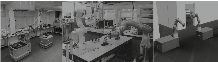
Fig. 4. (Left): Two KMR iiwa robots interacting with each other. (Centre): KMR iiwa placing the rack of vials in order for the Franka Emika robot to dispense liquid. (Right): two KMR iiwa robots interacting in Gazebo simulation environment.
