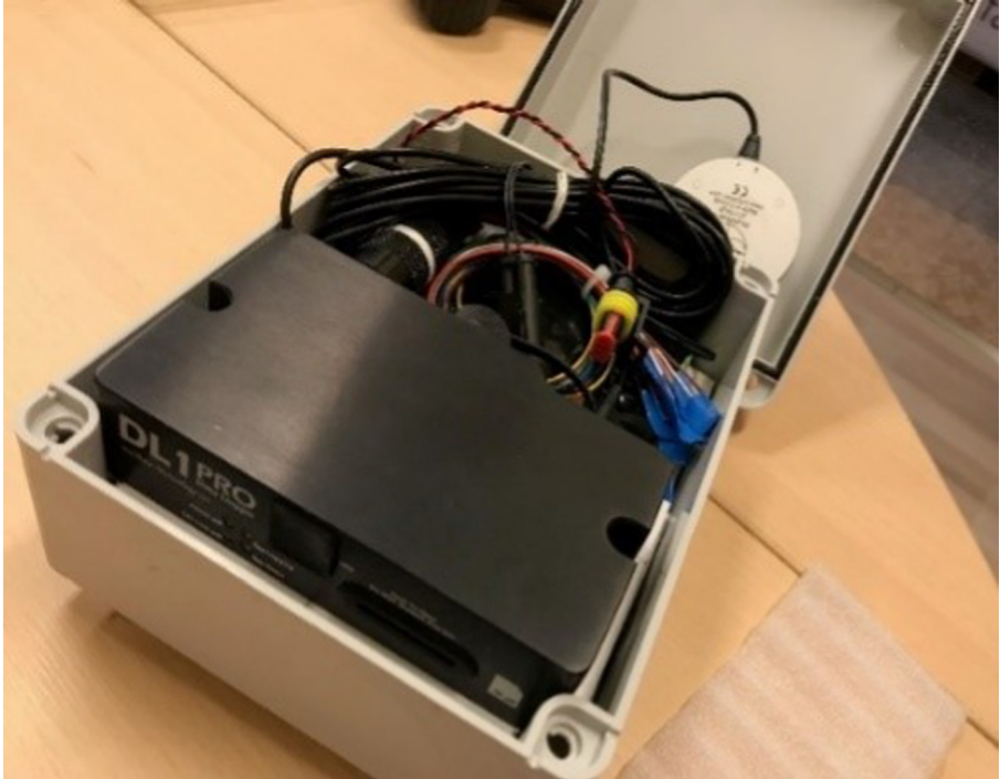
Fig. 1. Demonstration of the secured case with DL-1 MK2 Datalogger [11, 12].
