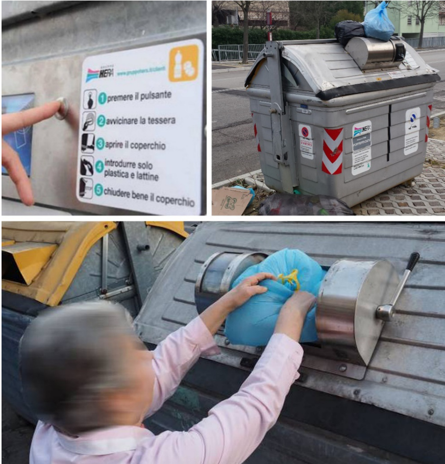
Fig. 1. The three main criticalities of standard volumetric cap: time-consuming process, with frequent mechanical disrupt and limited accessibility.
