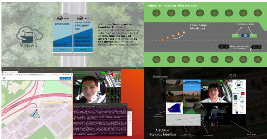
Fig. 2. Driver Monitoring System integrated into the VI-DAS vehicle, and demonstrated at the ITS Europe Congress 2019, with the DMS connected to the (Bottom-left) IoT solution and the decision making system (Bottom-right).
