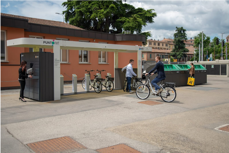
Fig. 13. Full-optional PUNTOnet station with parcel locker, e-bike sharing and smart waste containers. The shelter roof accommodates sensors and cameras previously packed in the smart totem.
