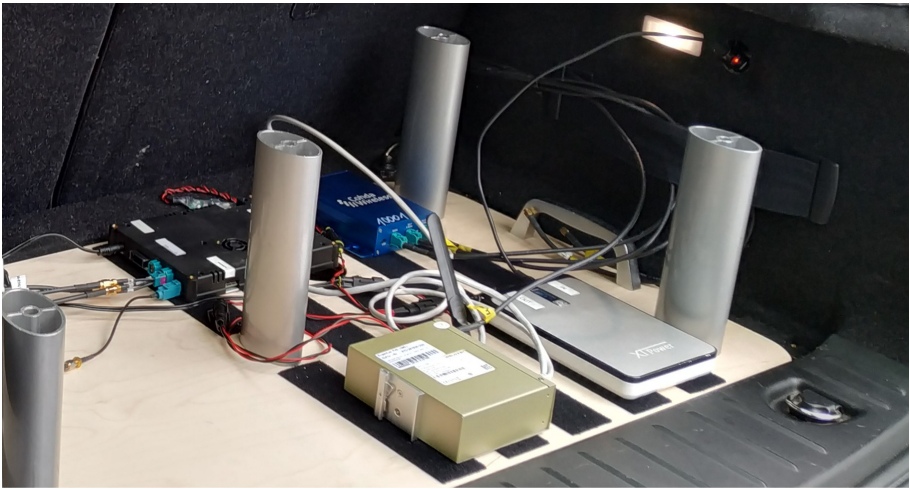
Fig. 3. Experimental setup for vehicles, consisting of Cohda MK5 (top right), C-V2X modem (top left), power supply (bottom right) and LTE router (bottom left). The equipment is installed in a BMW i3, but can be transferred to other vehicles.
