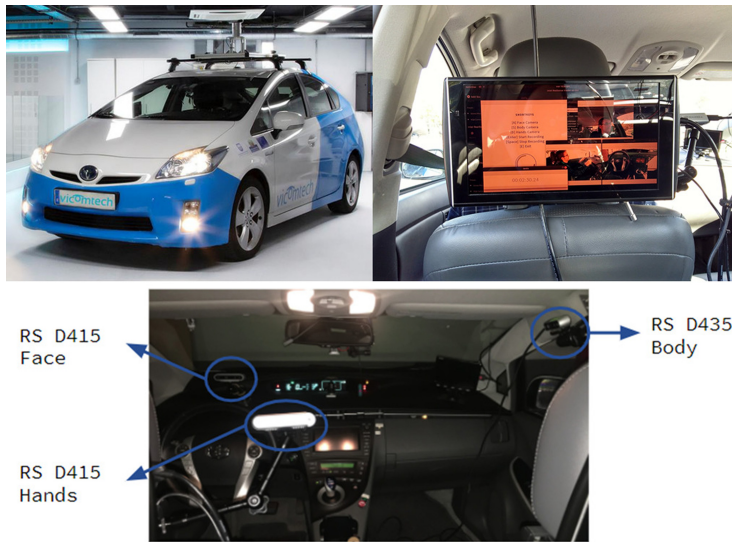
Fig. 10. Instrumented vehicle with interior cameras (Intel RealSense D400) for face, body and hands monitoring. The vehicle was instrumented also with perception and localisation devices (Velodyne HDL-32, 4 Sekonix 100° cameras, xNAV550, uBlox) and broadcasting mechanisms to send the output demo images to screens outside the vehicle.
