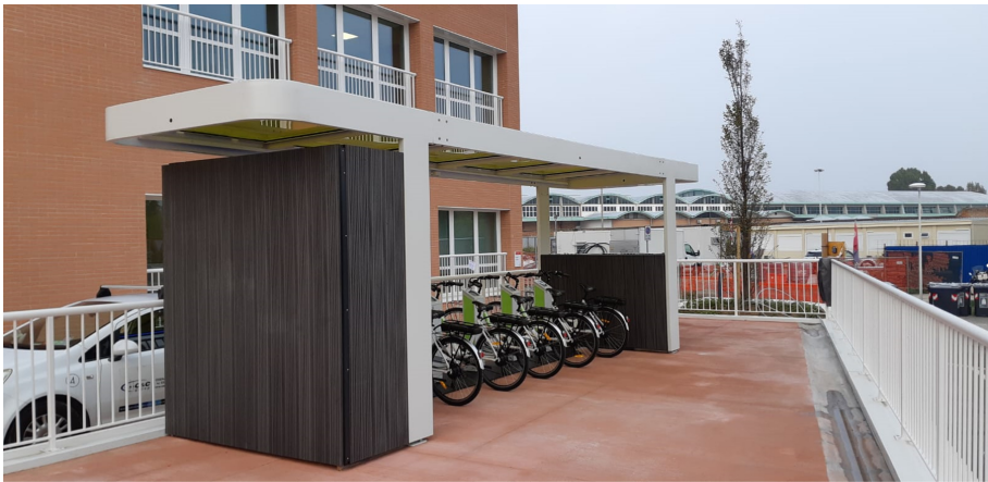
Fig. 12. PUNTOnet BIKE, with coloured photovoltaic glass, parcel locker and e-bike sharing system
