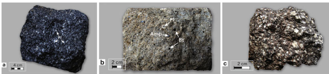
Fig. 4.1 Hand specimens of the Ciomadul dome dacites a dark grey dacite with glassy groundmass b light-coloured dacite with holocrystalline, light-coloured or felsic groundmass c brownish-red dacite with oxidized
