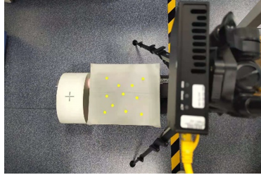
Fig. 3. RGB-D camera is placed nearly 73 cm above the breathing simulation. (Color figure online)
