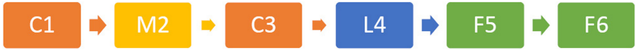
Fig. 2. Architecture of the proposed CNN. The CNN is composed of two convolution layers (denoted by C1, C2), two fully connected layer (F1, F2), max-pooling layer(M) and a locally connected layer (L).
