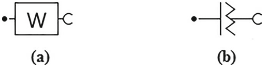
Fig. 6 a Warburg impedance, b Constant phase Element, other circuit elements used for the fitting of EIS data
