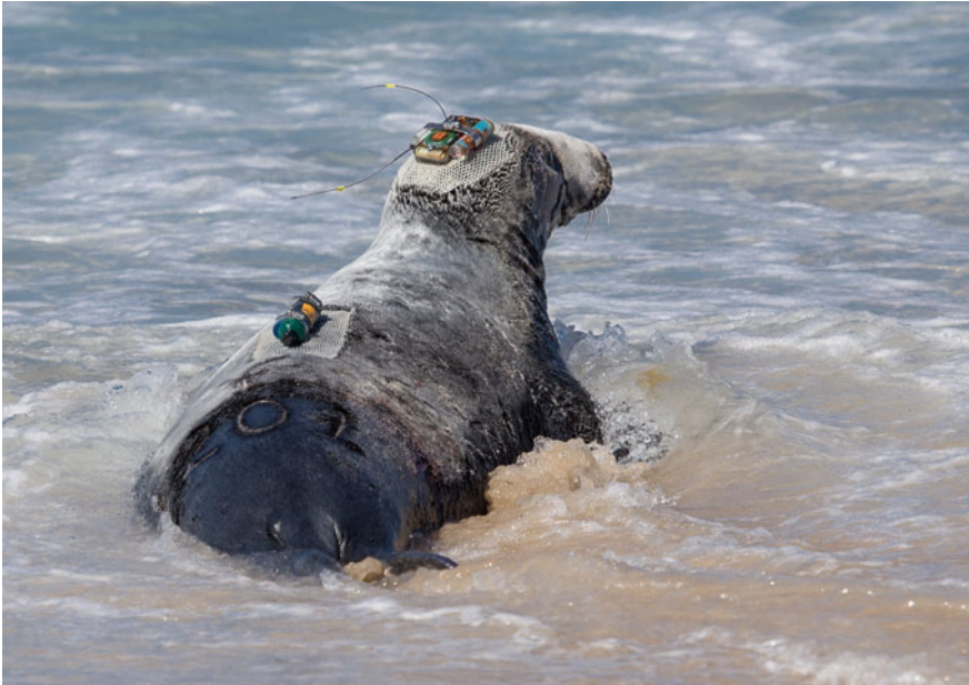
Fig. 6.7 A 30-year-old female gray seal fitted with a satellite-linked/GPS, time-depth recorder tag, a VHF radio tag, an accelerometer (head-mounted) and an acoustic transceiver (back) to study temporal and spatial encounters with acoustically tagged prey species. Photo by W. D. Bowen
