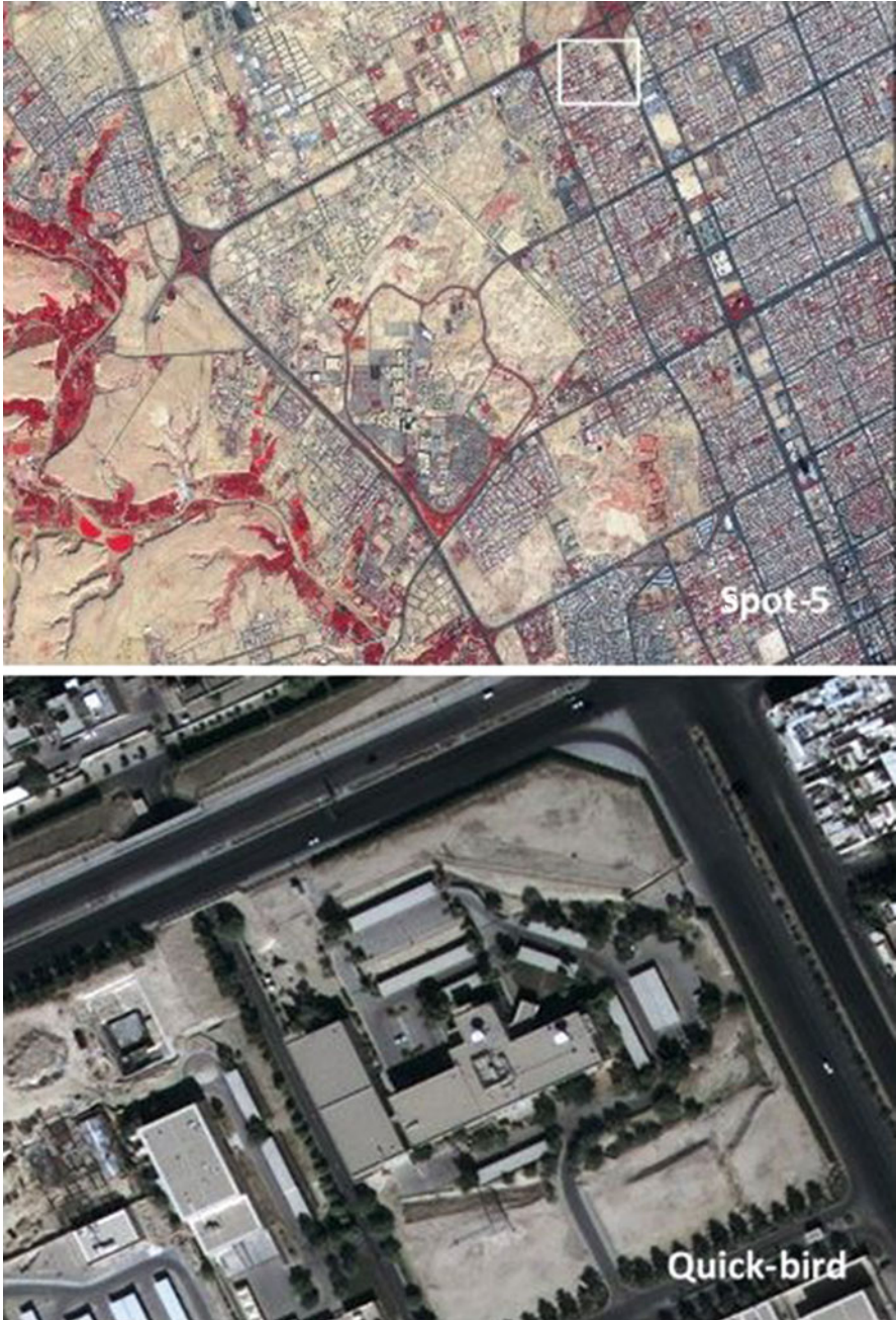
Fig. 1.2 Satellite images with different spatial resolution (Spot-5 with 5 m and Quick-bird with 0.61 m; the Quick-bird image is indicated in the white frame above in the Spot image)
