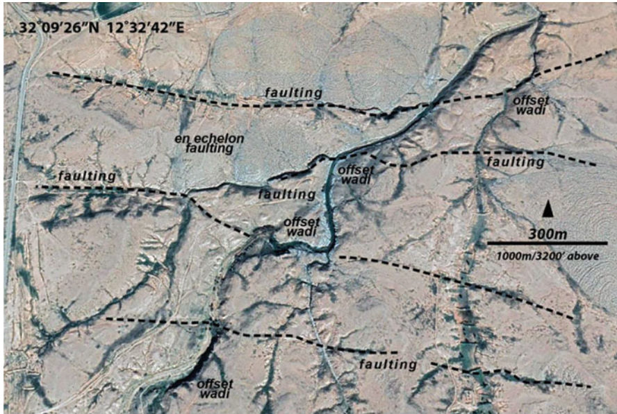
Fig. 24.5 Matched image displaying (a) en-echelon faulting, (b) faultings, (c) and offset wadi channels located in 32°09' N 12°32' E northeast Al Jabal Al Gharbi western Libya (Google Earth, 2019a)
