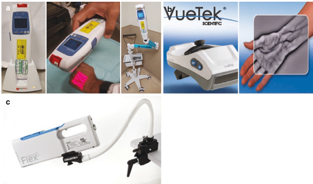
Fig. 12.6 Examples of the infrared vein viewing devices. (a) Accuvein, (b) Veinsite, (c) VeinViewer
