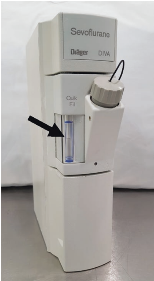
Fig. 5.8 Example of an anaesthesia vaporiser for Sevoflurane. Photo demonstrating an adequate level in the window chamber (arrowed)
