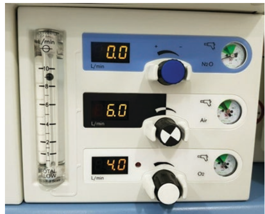
Fig. 5.7 Hypoxic guard proportioning system. The automatic adjustment of oxygen when Nitrous oxide flow is increased to prevent a hypoxic gas mixture
