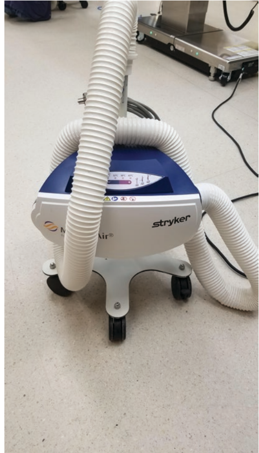
Fig. 13.4 Stryker air conduction warming system. Blower. It enables warming at two different temperatures plus cooling (32 °C)
