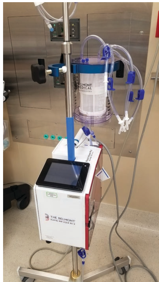
Fig. 13.1 Belmont Infusion system. This system consists of several components that are reusable and disposable. Requires priming with a primer solution (electrolyte solution, colloid or blood product)
