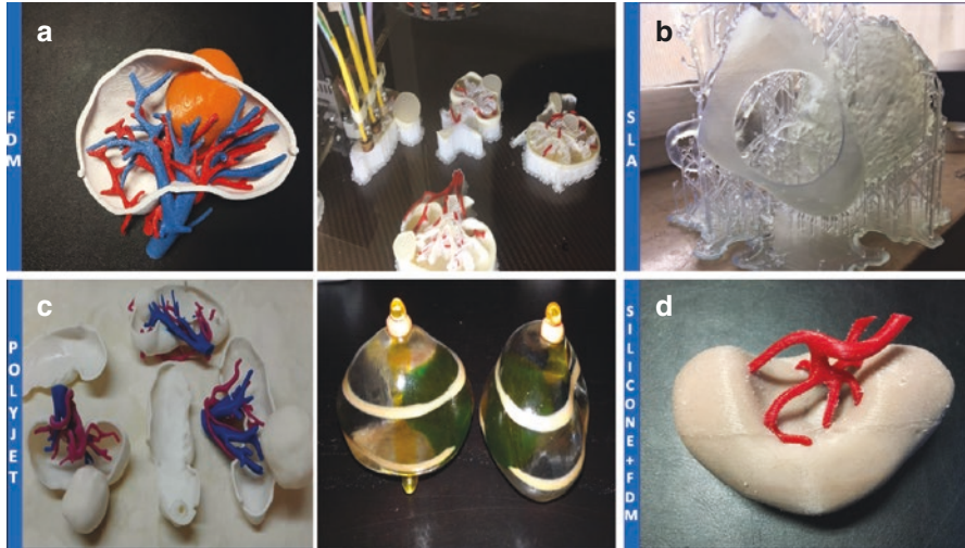
Fig. 26.2 Different 3D printing technologies: (a) Fused Deposition Modeling (FDM); (b) Stereolithography (SLA); (c) Multi-material Plastic Jetting (Polyjet); (d) Silicone mold pouring combined with FDM printing
