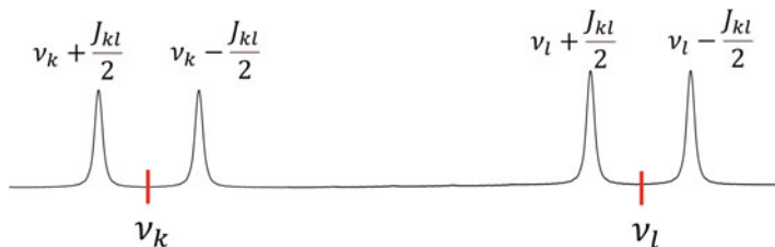
Fig. 5.7 A schematic of the J-coupled spectrum for a two-spin system, where \nu_k and \nu_l are the frequencies of k and l spins, respectively, and J_{kl} is the J-coupling between k and l spins
