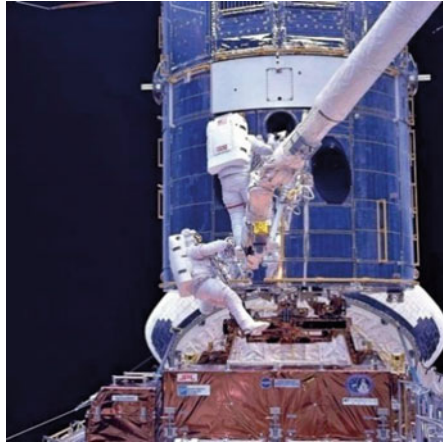
Fig. 25.2 Servicing mission SM1 (STS-61) for the Hubble Space Telescope, during which corrective optics were installed in December 1993 ( Credit NASA )
