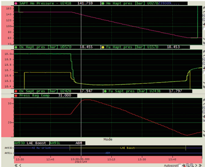
Fig. 21.3 Pressure development during AMF2. The first graph above shows the pressure in the helium tank. The second diagram shows the pressures in the two tanks for oxidizer (U057D in green) and fuel (U157D in yellow). The third graph shows the temperature of the pressure regulator and the last graph above represents the state of the attitude and orbit control system (AOCS) software and shows when the orbit maneuver takes place
