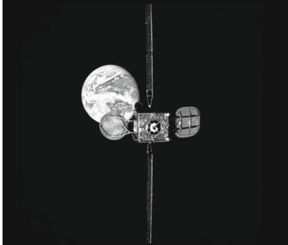
Fig. 25.5 View of target satellite in GEO from MEV-1’s “far hold” position during approach from approximately 80 m with Earth in the background ( Credit Northrop Grumman )
