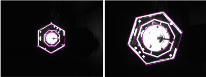
Fig. 25.20 The images from a mono camera from two different distances are overlaid with the result of the image processing (projected 3D model of the target in magenta color)
