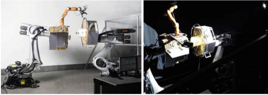
Fig. 25.27 On-orbit servicing simulator (OOS-Sim)—a test facility for capture maneuvers operations located at the Robotic and Mechatronic Center in Oberpfaffenhofen ( Source DLR)
