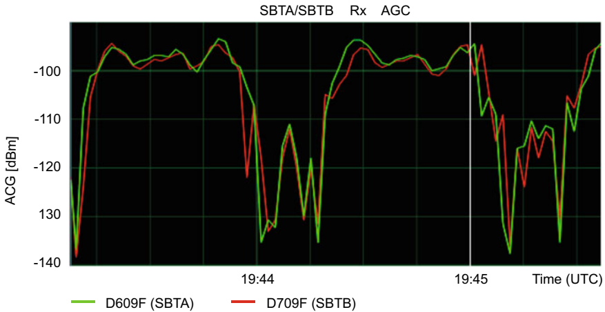
Fig. 6.15 On-board AGC of S-band receiver A (D609F) and B (D709F)
