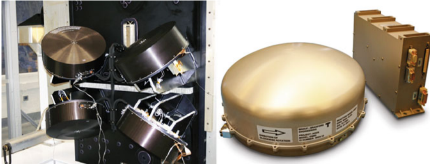
Fig. 22.5 Left: Reaction wheels on Lunar Reconnaissance Orbiter, NASA GSFC (image: NASA); right: Reaction wheel unit (image: bradford-space.com)
