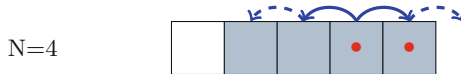
Fig. 4. A stream execution of length N+1 with the corresponding template unfolding is depicted. The stream execution covers all cases where future out-of-accesses occur. Gray-colored and red dotted positions represent unfolded assumptions and assertions, respectively. Solid and dashed arrows indicate accesses by streams and annotations, respectively. (Color figure online)
