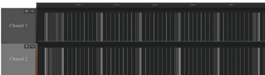
Fig. 37.7 The result obtained by recording the communication 60 s: channel 1. is TX signal, channel 2. is RX signal
