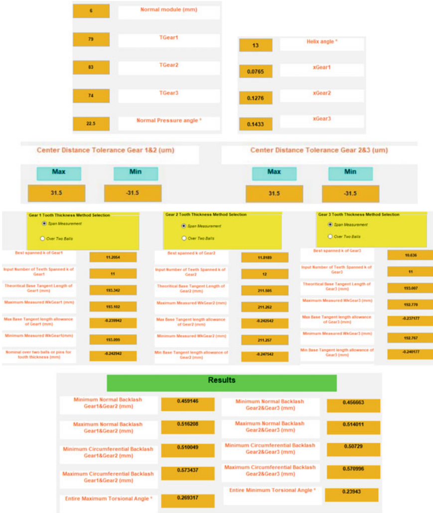
Fig. 6.2 Self-compensated backlash gear train program under case study
