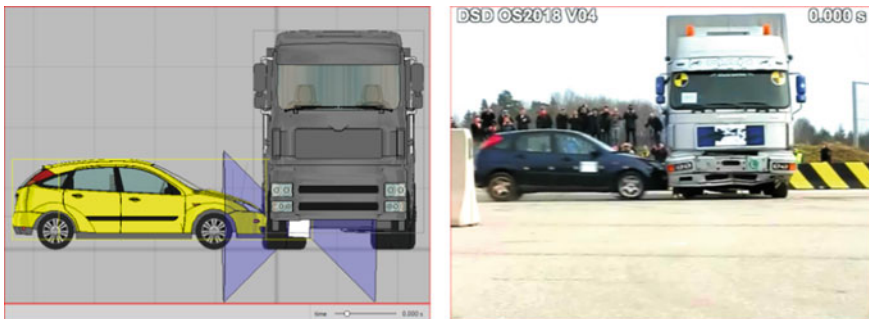
Fig. 43.3 First contact (at t = 0.000 \text{ s} in the simulation-left, real test collision-right [5])
