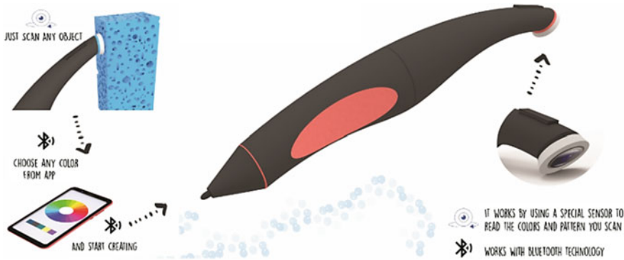
Fig. 76.2 “Pigmentum”—Concept of a device that can scan color and pattern from objects, shaped as a leech to express a simple association to its functionality (student project)
