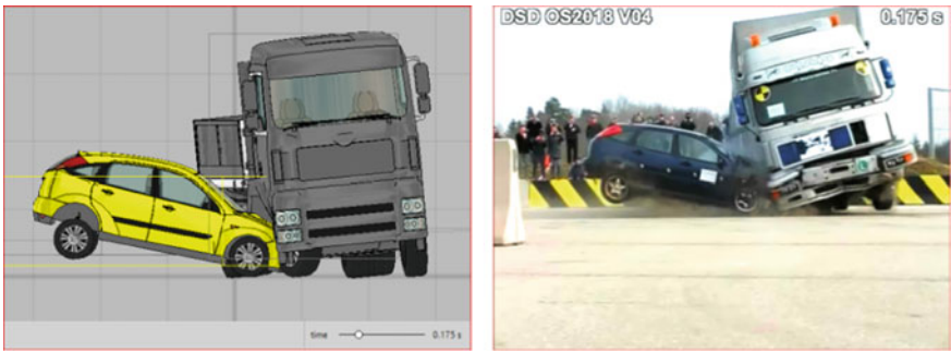
Fig. 43.5 Positions at time t = 0.175 s (simulation-left, real test collision-right [5])
