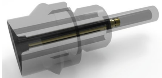
Fig. 18.4 Creation of the working surface of the tool-valve applicator
