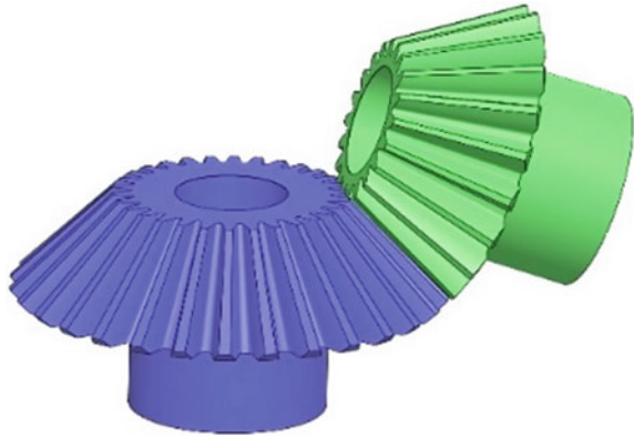
Fig. 7.3 A CAD assembly models of a bevel gear pairs by SolidWorks software ( \Sigma = 70^\circ )
