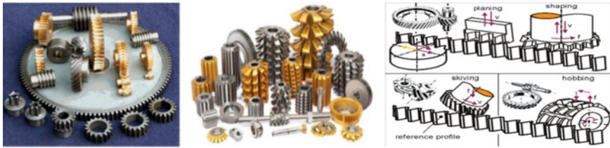
Fig. 24.1 Basic forms of serration, basic gear cutting tools and gear cutting methods
