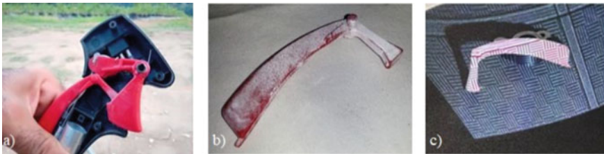
Fig. 56.1 a Gas handle, b matting gas handle and c 3D scanning of the handle
