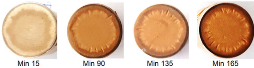
Fig. 29.2 The evolution of the eroded area according to the cavitation exposure duration (recorded with a Canon A480 camera)
