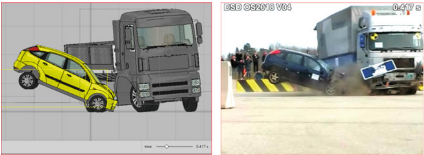
Fig. 43.6 Positions at the moment t = 0.417 s (simulation-left, real test collision-right [5])
