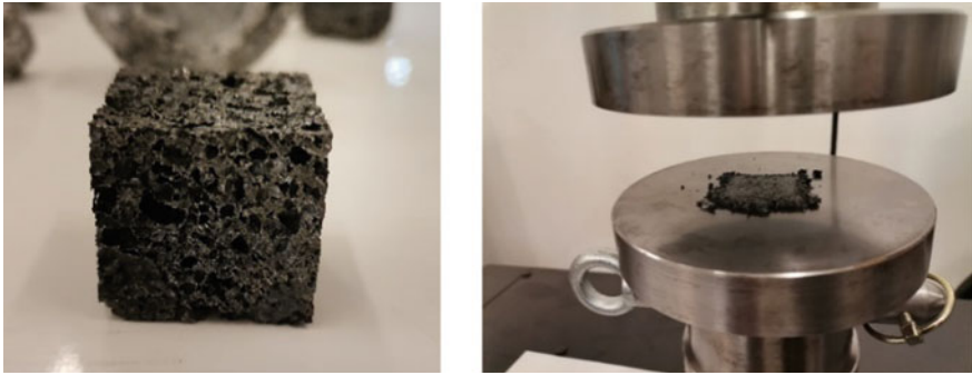
Fig. 28.4 A sample and a compressed foam in the testing apparatus
