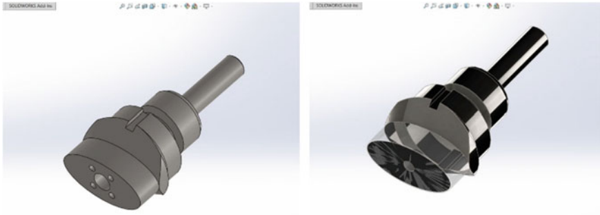
Fig. 18.4 Creation of the working surface of the tool-valve applicator
