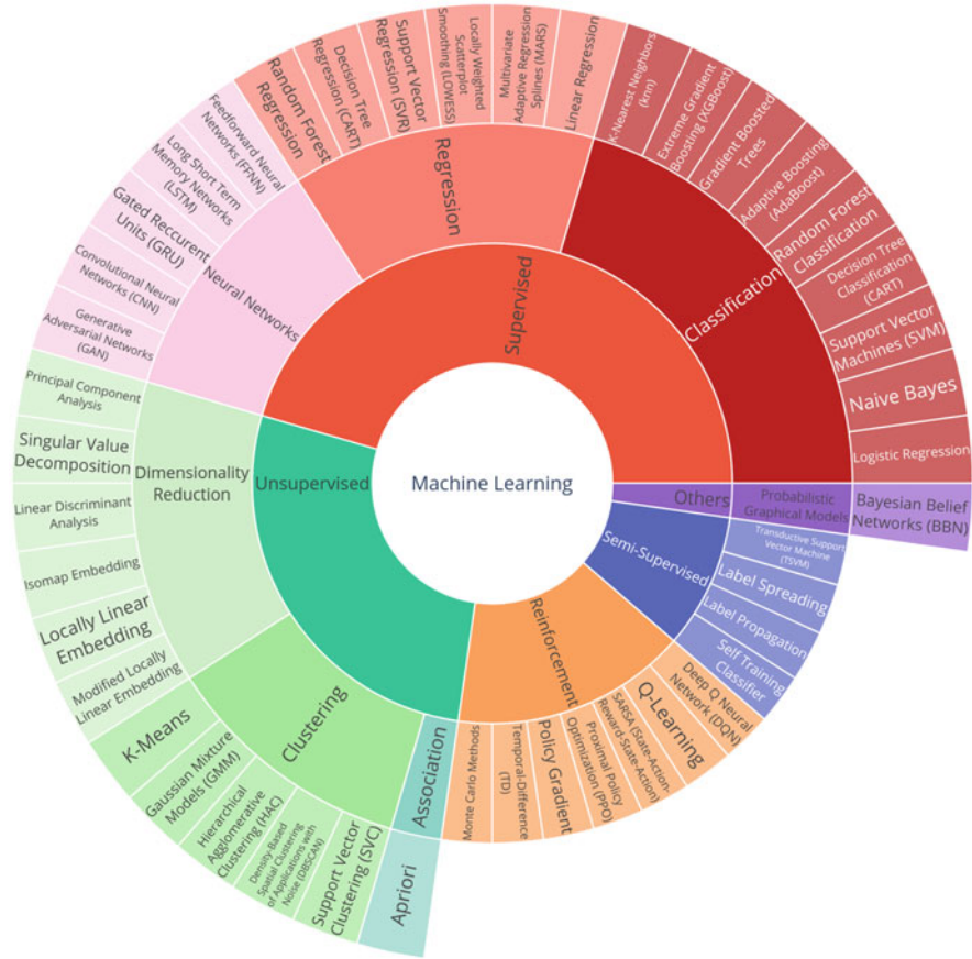
Fig. 4 Machine learning paradigms and algorithms. (An interactive version of this figure is available at: http://www.datascience-in-tourism.com/?p=132 ). Source: Dobilas (2021)
