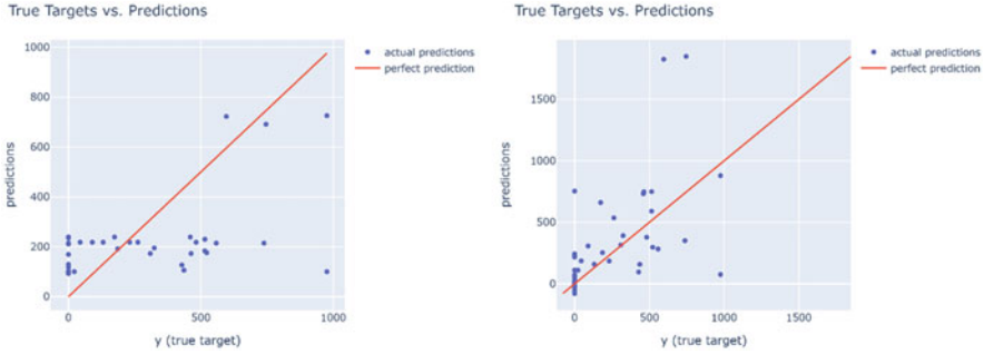
Fig. 9 Scatter plot that contrasts prediction and true values for random forest (left) and gradient tree boosting (right); both models were trained with all nine features
