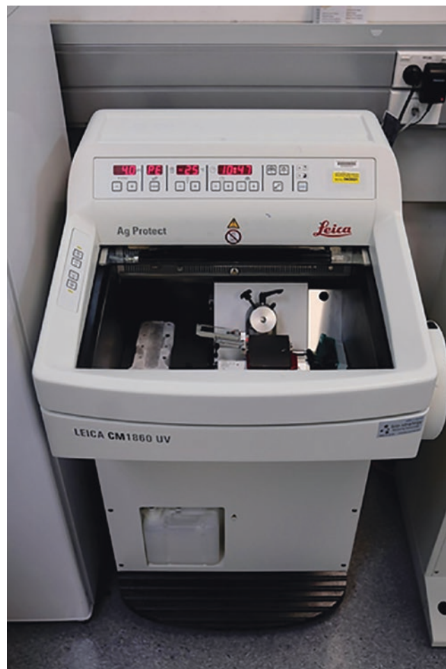
Fig. 8 Leica™ CM1860UV cryostat machine, used for cutting frozen sections either in theatre or in the laboratory
