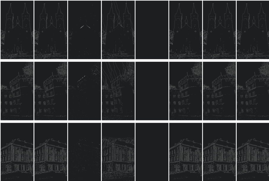
Fig. 11. ED results on natural image dataset. Columns: Sobel, Prewitt, Kirsch, Kitchen, Kayyali, Scharr, Kroon, Orhei
