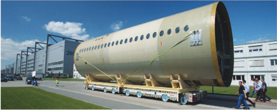
Fig. 16.10 Fuselage section made up of composites for the A350 XWB in Hamburg, Germany (Marsh, 2010)
