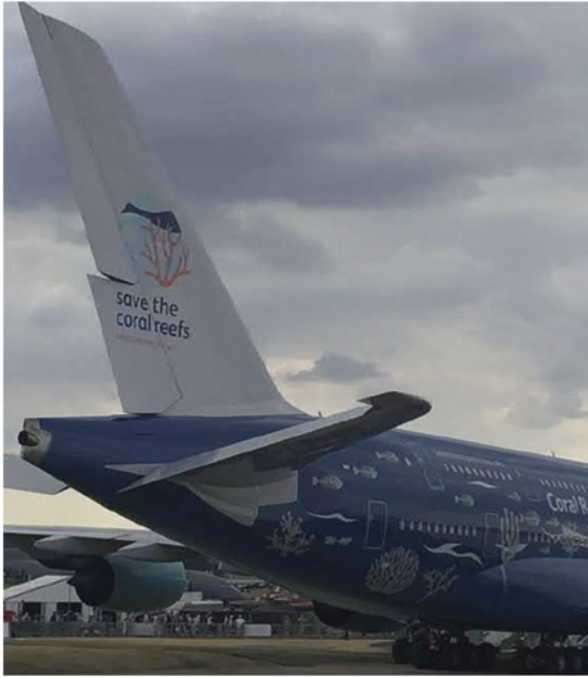
Fig. 16.7 A380 composite tail assembly (empennage) with glare fuselage crown (Soutis, 2019)
