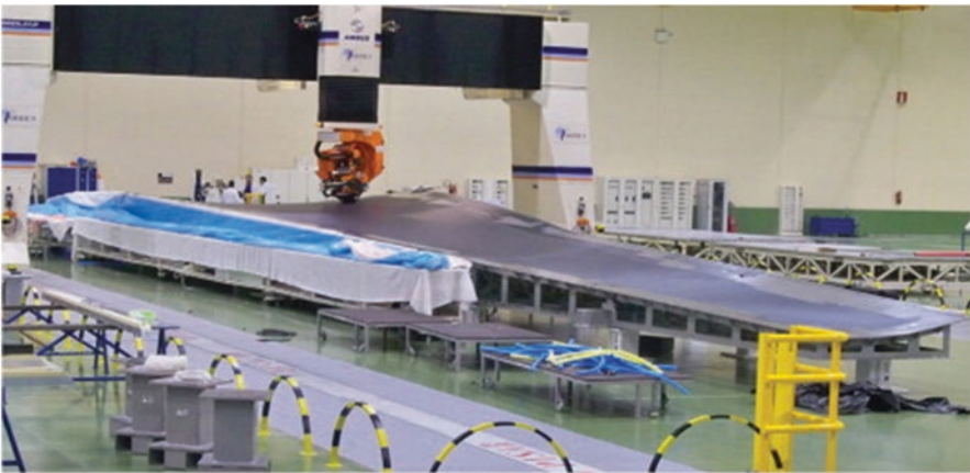
Fig. 16.11 Manufacture of lower wing shells of A350 XWB model (Marsh, 2010)
