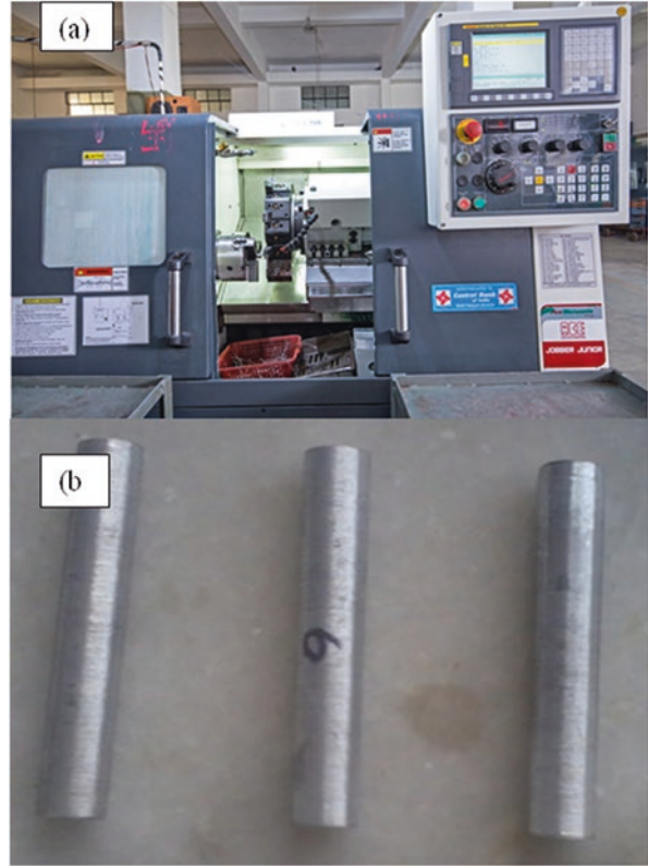
Fig. 12.4 (a) Experimental set-up for CNC lathe machine used for turning of the specimens and (b) machined samples
