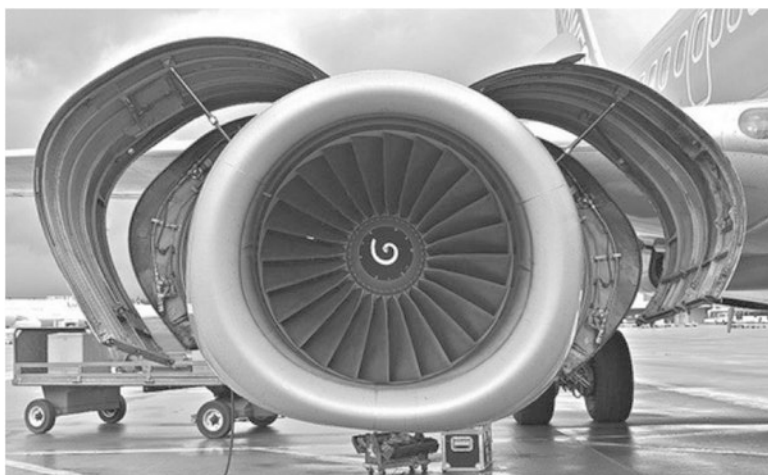
Fig. 16.8 Gas turbine engine nacelle and cowling made up of composite material (Mouritz, 2012)
