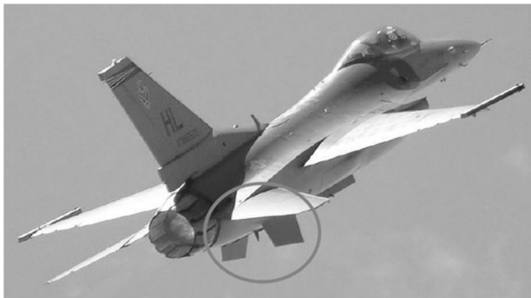
Fig. 16.12 Aluminum-SiC composites utilized in the ventral fins (circled) and fuel access doors of the F-16 Fighting Falcon (Mouritz, 2012)
