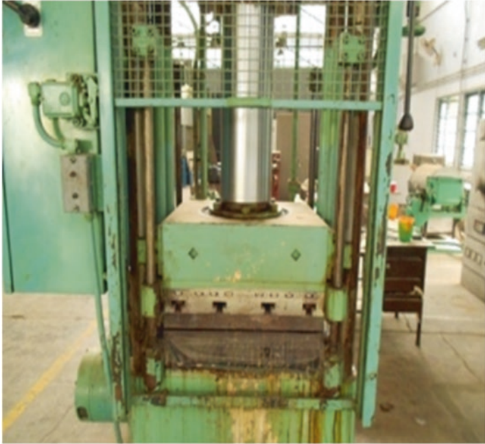
Fig. 2.6 Compression molding machine used for making laminates
