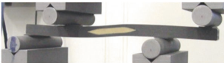
Fig. 4.7 Coupon test set up with embedded foam insert
