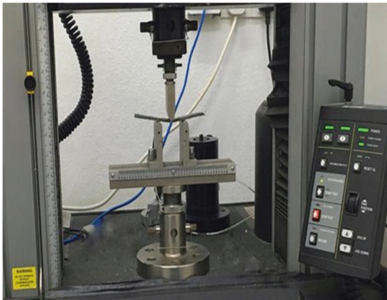
Fig. 17.6 Three-point bending test on fiber-reinforced PLA nanocomposite
