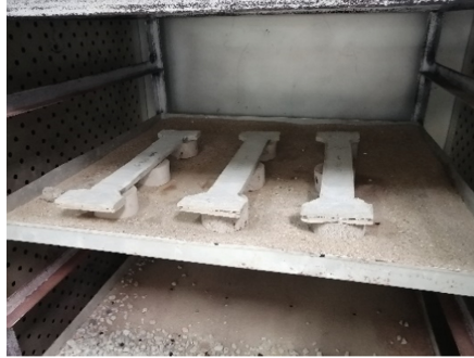
Fig. 2. TRM coupons inside the heating chamber.
