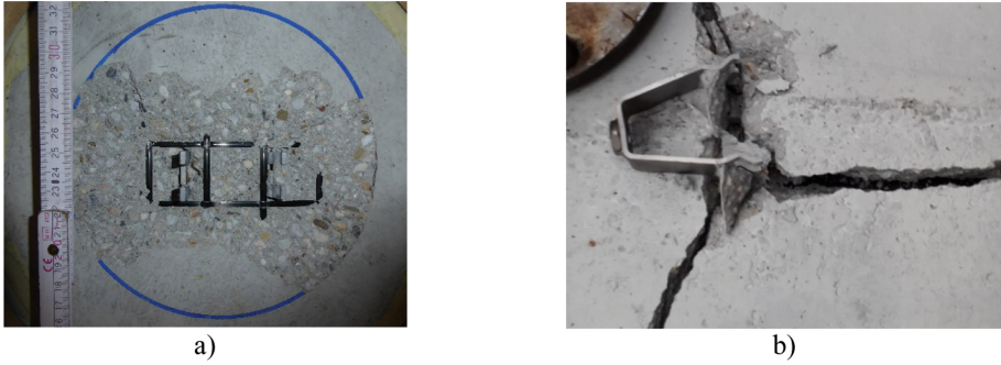
Fig. 12. a) Concrete rapture cone of a compression test with CFRP reinforcement reinforced panel ( 1.8 \text{ m} \times 1.8 \text{ m} ), b) Tensile test with concrete panel ( 0,5 \text{ m} \times 0,5 \text{ m} ) without reinforcement.
