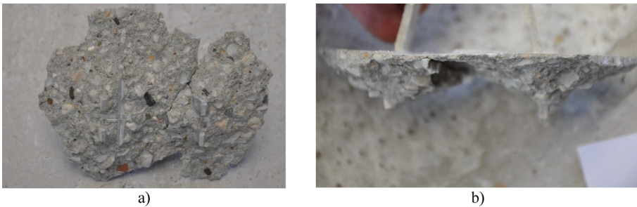
Fig. 11. Concrete rapture cone of a tension test with CFRP reinforcement a) side view, b) front view.
