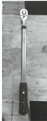
Fig. 7. Torque wrench with controlled tightening.
