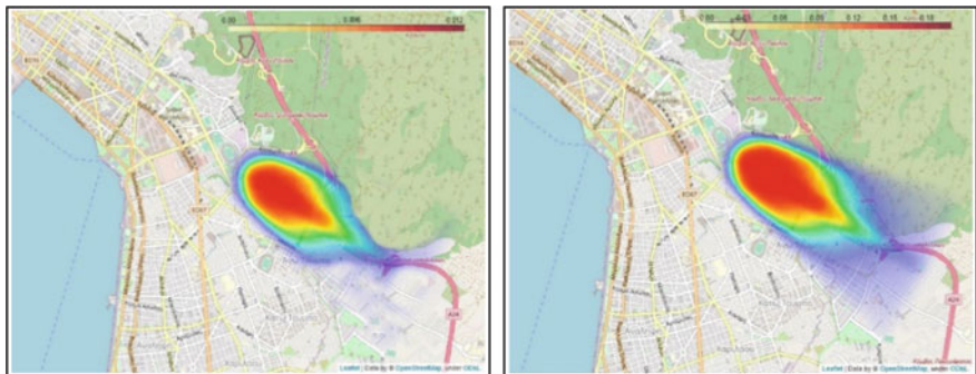
Fig. 7 Heatmap of NO x concentration for Department of Architecture in scenario 2 (left: natural gas emissions, right: heating oil emissions). Differences in focal point of high concentrations are located in variations of red color which displays the maximum values. In the case of heating oil, we have darker shades of red compared to the ones of thematic map of natural gas
