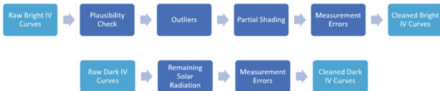
Fig. 4 Steps in the Cleaning-Pipeline for the raw bright (top) and dark (bottom) IV string curve data
