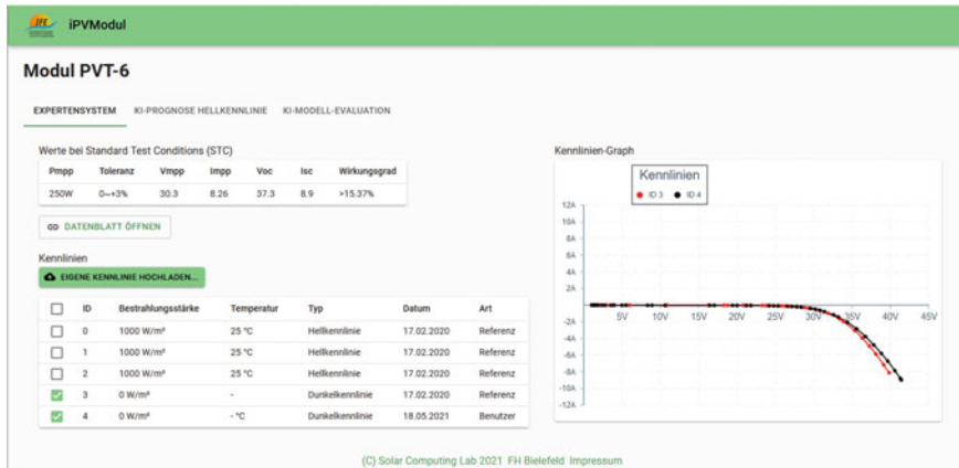
Fig. 11 Comparison of historical dark IV curve data in the web-database-application iPVModule
