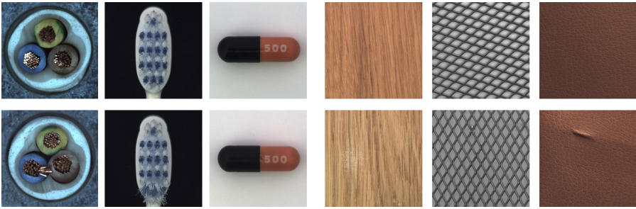
Fig. 3. Object (cable, toothbrush, capsule) and texture (wood, grid, leather) images in MVTEcAD [2]. The images in the upper row are normal samples and the ones in the lower row are abnormal samples.
