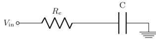
Fig. 1. Electric diagram of the series Resistor-Capacitor (RC) circuit. The circuit is composed of a voltage supplier V_{in} , a resistor R_e that is analog to the excitatory synapses of the neuron and a capacitor C that reproduces the membrane potential.
