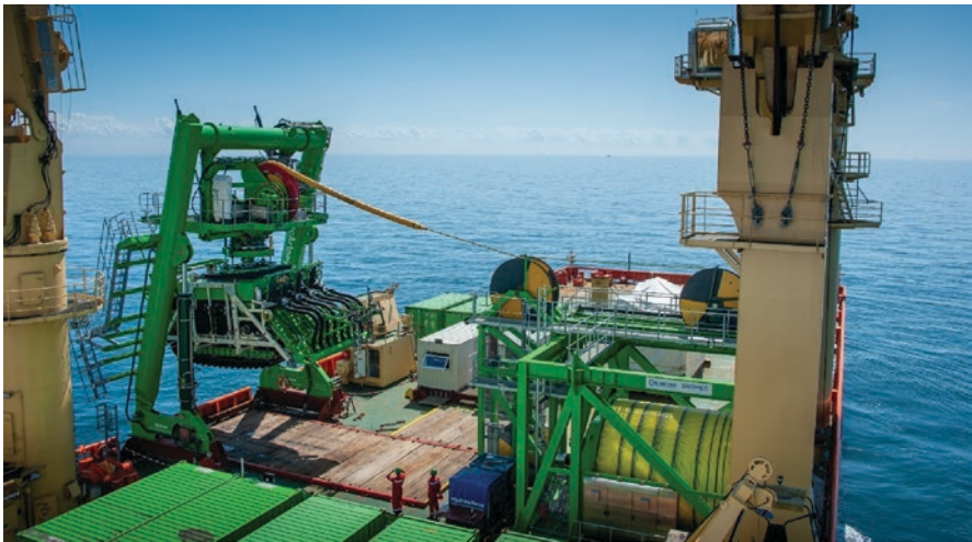
Fig. 6.15 PATII's launch and recovery system (A-frame and umbilical winch) (July 2020)
