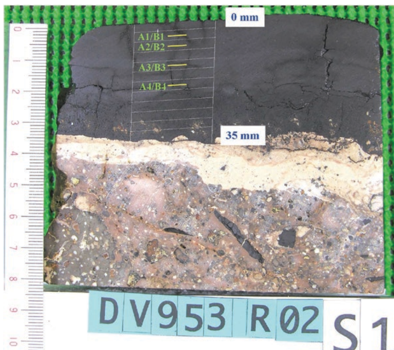
Fig. 5.1 Cross-section of the studied ferromanganese crust (35 mm thick) on phosphatized limestone and altered basalt. A monotonous structure of earthy black compact layers is observed
