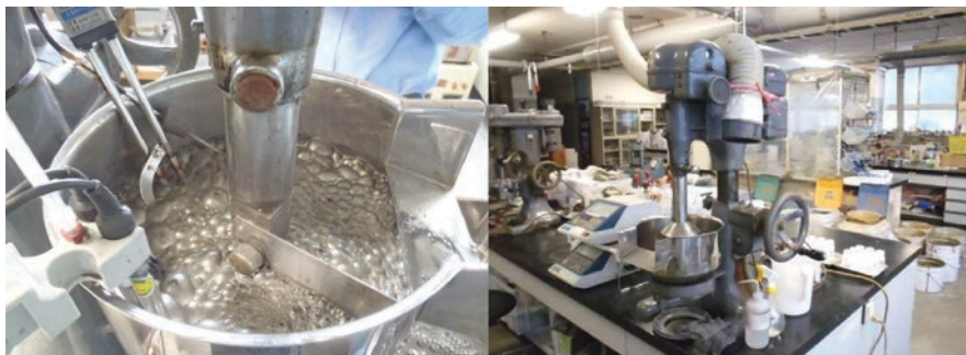
Fig. 7.22 Lab flotation test equipment
