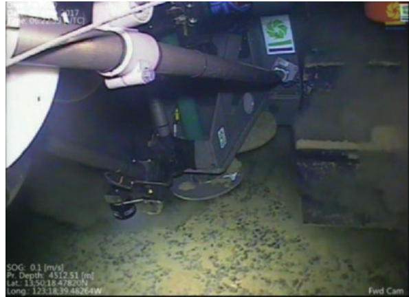
Fig. 6.3 Pressure plates mounted on Patania I (June 2017)
