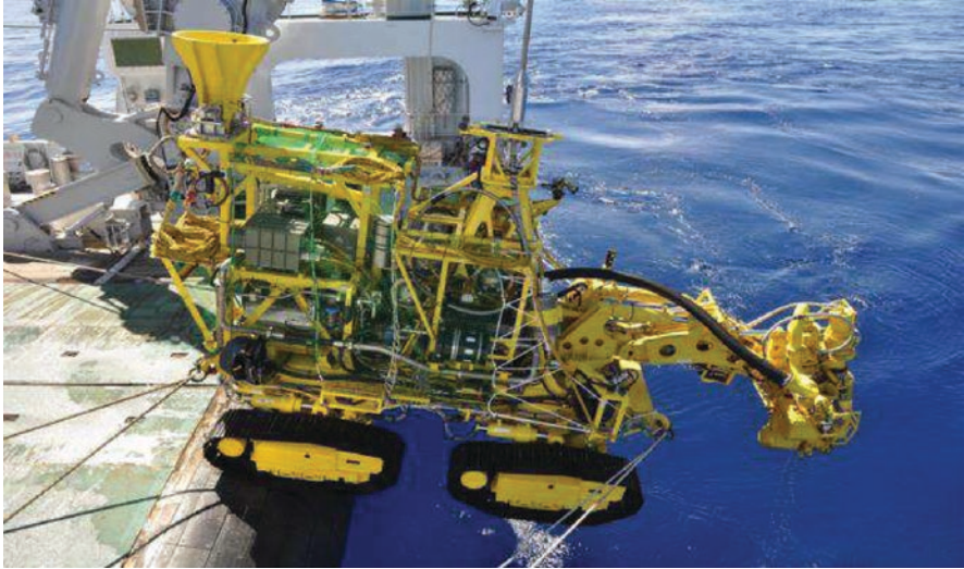
Fig. 7.10 Ore-collecting test machine launched from the deck of “Hakurei” (METI 2017; Okamoto et al. 2019)
