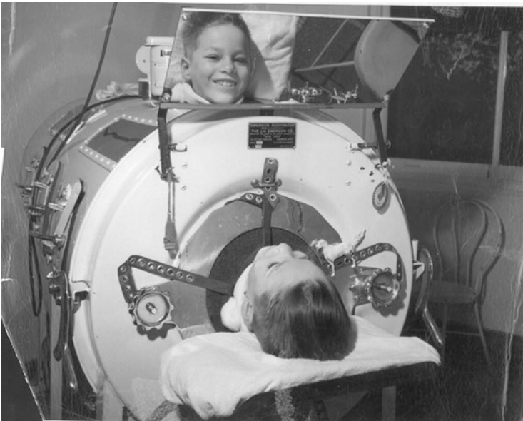
Fig. 3.1 The Emerson respirator, more commonly known as an “iron lung.” Photo credit: “NCP4145” by otisarchives4 is licensed under CC BY 2.0
