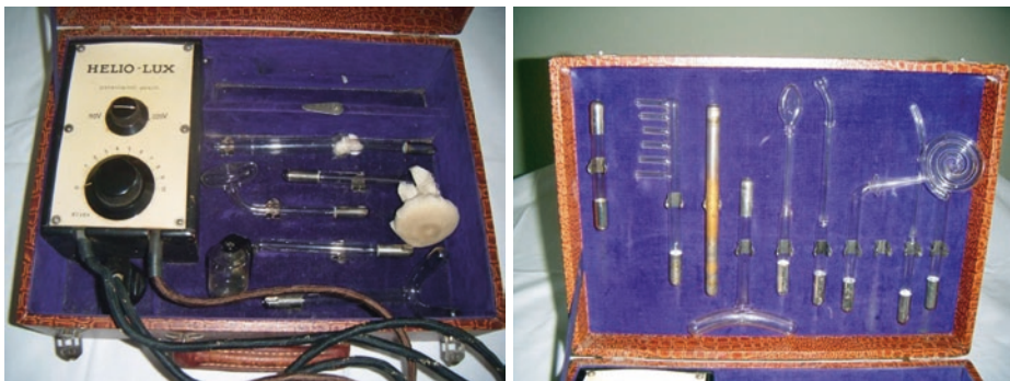
■ Fig. 4.2 Suitcase containing control unit as well as set of glassy vacuum electrodes of the antique HELIO-LUX high frequency (HF) apparatus. (Picture source: Ramona Meißner-Kellotat, Medical Historic Collection of the Institute of Ethics and History of Medicine, University Medicine Greifswald, Germany)
