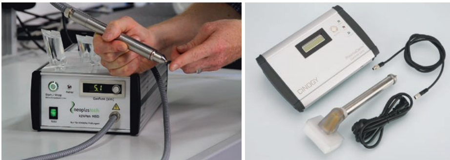
■ Fig. 1.10 The plasma jet kINPen® MED by Neoplas tools GmbH, Greifswald (left) and the DBD plasma source PlasmaDerm by Cynogy GmbH Duderstadt (right). (These figures have been published in: Comprehensive Clinical Plasma Medicine – Cold Physical Plasma for Medical Application , Springer 2018, p. 140)
