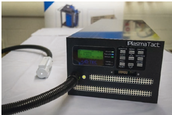
■ Fig. 18.5 The portable PlasmaTact cold plasma device with its handheld plasma-pen style design
