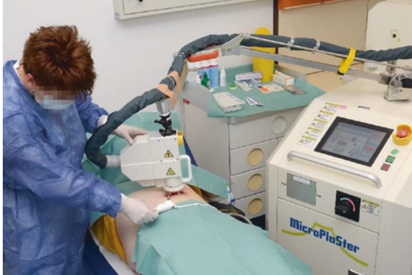
■ Fig. 18.3 The Adtec MicroPlaSter: Adtec's first CE-certified cold plasma medical device in use at a German hospital
