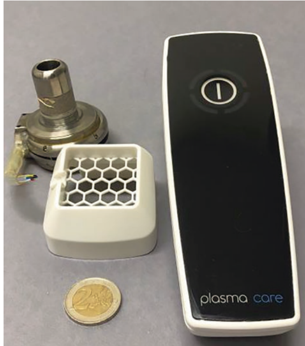
■ Fig. 12.1 Model of a modified spacer for the plasma care device for plasma application in VAD, ADC, and PDC patients
