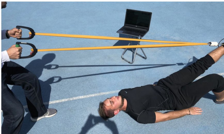
Fig. 3 DINABANG is a portable instrument to measure force and speed (hence power) involved in lower limb rehabilitation or training. Either excess or lack of effort may lead to lesions or ineffective training or rehabilitation. DINABANG fulfills the need to quantify effort during exercise, in the sports field
