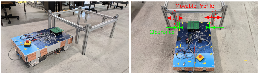
Fig. 9. Experimental setup with SLAMdog. The profiles (marked with red dashed boxes) can be adjusted according to the experiment requirements for the clearance. (Color figure online)
