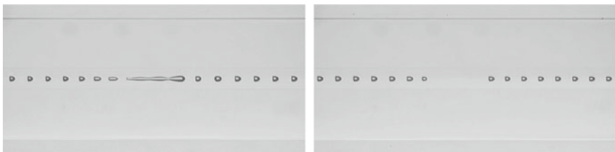
Fig. 7.8 Photographs of irregular segments left at the decrement (left) and increment (right) points of the pump power. Fiber: SMF-28e, laser: 1480 nm, 6.5 \rightarrow 5.6 W (left) and 4.9 \rightarrow 5.5 W (right) (Reprinted with permission from [4]. © 2014 NIMS)
