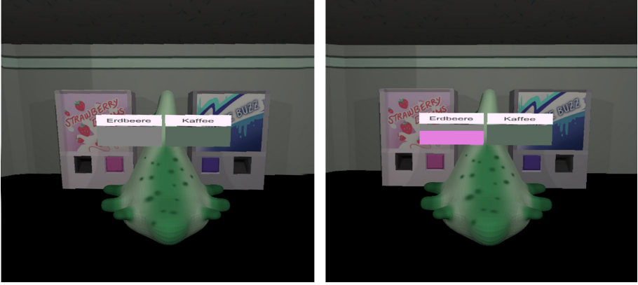
Fig. 4. Button method: The gaze button fills from the bottom while looking at it, in this case the left button. When the button is filled completely the decision is done.
