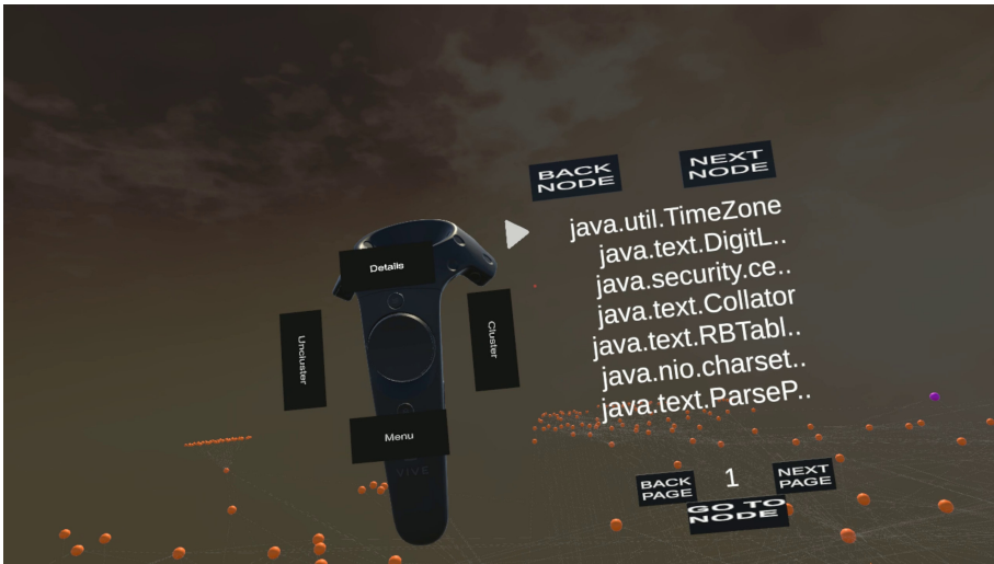
Fig. 6. The application menu. On the controller mesh the Cluster , Uncluster , Details , and Menu buttons appeared. The user can interact with them to perform the clustering, unclustering, view node or cluster details, and close the menu. The image on the right shows how to consult the list of selected nodes. The user can select a node from the list and teleport in front of the desired node through the Go To Node button.
