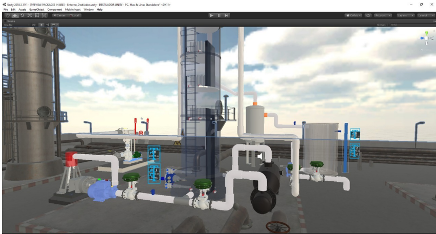
Fig. 8. Binary distillation tower design based on the P&ID diagram.
