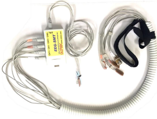
Fig. 2. Low-cost wearable EEG acquisition system.
