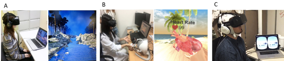
Fig. 3. A. A virtual reality world watched by the participant through the Oculus Rift; B. A biofeedback based VR-haptic system; C. A neurofeedback based immersive VR solution.
