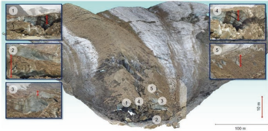
Fig. 5.12 Areas identified for comparison of point clouds from UAV, terrestrial photogrammetry, and laser scanning acquired in 2016 (Fugazza et al., 2018)
